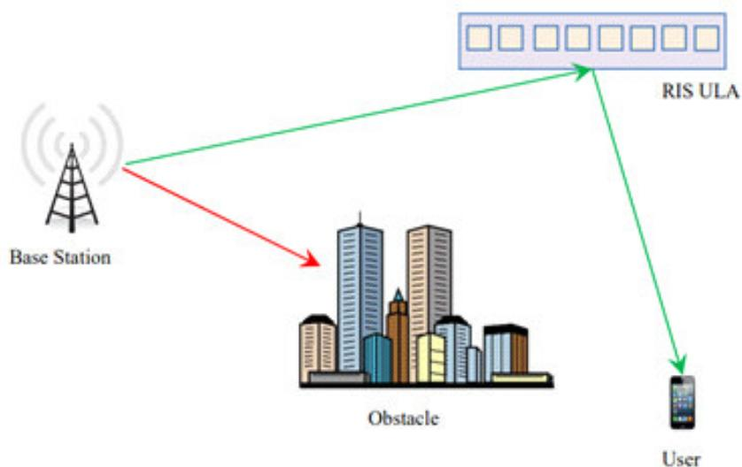
**Figure 1 Reconfigurable intelligent surface assisting BS to connect to the user.**
